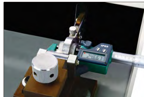
lapping measuring surfaces of outside micrometer
