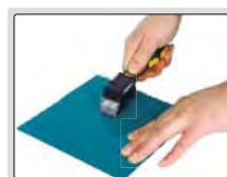
step 1: make grid cutting on surface
