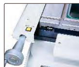
X-axis reset switch
