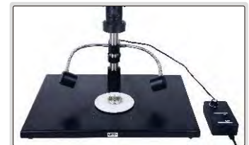
illumination direction and brightness are adjustable
