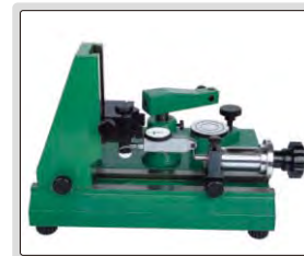
inspect accuracy of test indicators
