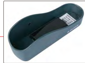
base with calibration block (included)
