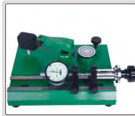
inspect accuracy of dial indicators (range 0-25mm)
