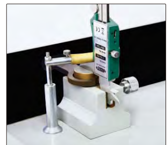
lapping measuring surfaces of caliper lower jaws
