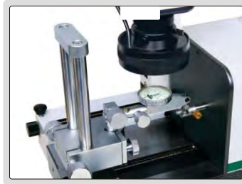
check dial test indicators
