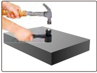
hammer impact to apply test force
