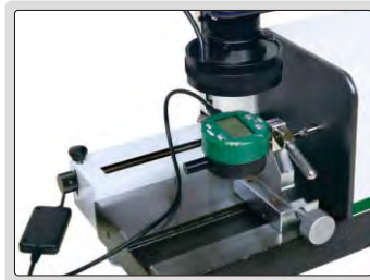
check INSIZE digital indicators (connection with cable)
