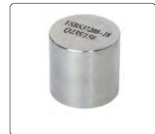
15# carbon steel control sample (optional)
